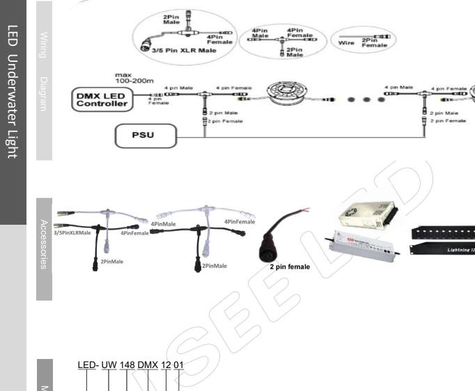
01=Pixel Quantity 12=LED Quantity DMX=Control Protocol 148=Diameter(mm) UW=Underwater LED=ISEELED
